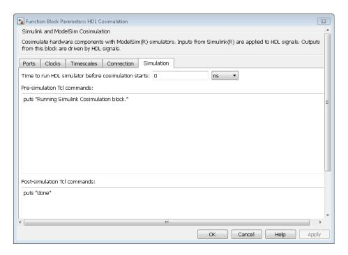
You may specify any valid Tcl command string. The Tcl command string you specify cannot include commands that load an HDL simulator project or modify simulator state. For example, the string cannot include commands such as start, stop, or restart (for ModelSim) or run, stop, or reset (for Incisive).
