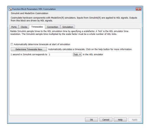
The **Timescales** pane specifies a correspondence between one second of Simulink time and some quantity of HDL simulator time. This quantity of HDL simulator time can be expressed in one of the following ways:
